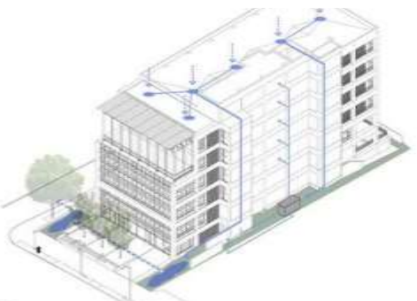
Perkins & Will Office Rainwater Harvesting System Source: http://perkinswill.com/ (Accessed on 27 th December 2015)
