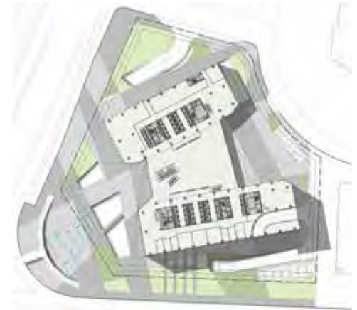
Figure 9. A first level floor plan, illustrating how activity at the ground level is promoted by a unified lobby experience. (Source: NBBJ)
