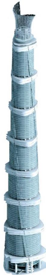
Figure 3.1. With the outer skin removed, the regular circular floor plates are revealed. (Source: Gensler) 图3.1. 将外层表皮剥离后, 可以看到每层平面都呈现规则的圆形。(来源: Gensler)
