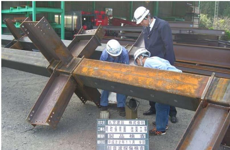
Ultrasonic Test Inspection
